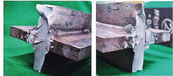
[Overhead: AFR (LTTB)-6-O/H (150 N/mm 2 , 1.35 \times 10^6 cycles)]
