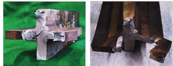
[Vertical Upward: AFR (LTTB)-8-V/U (150 N/mm 2 , 2.66 \times 10^6 cycles)]
