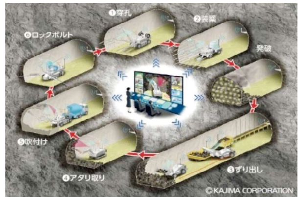
図-8 A 4 CSEL for TUNNEL 7)
